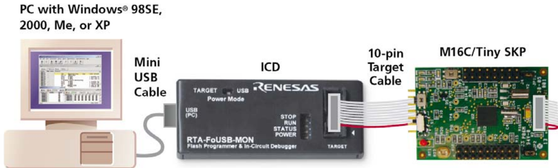
Figure 4-1 SKP16C28 FLGA System Connectivity
